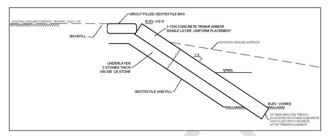
Figure 3: Alternative 2 – Tribar Revetment
