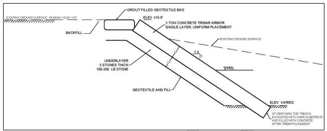
Figure 2: Alternative 2 - Tribar Revetment
