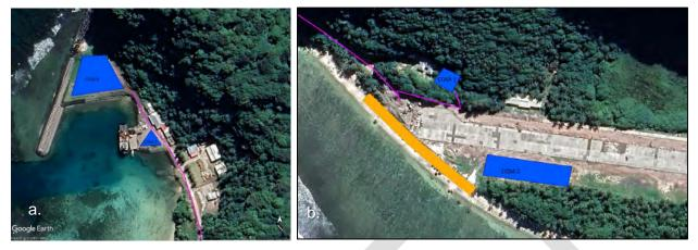
**Figure 4.** The proposed Action Area includes four Construction Staging Areas (COSAs) in blue: a. COSA 3 and 4 at Ofu Harbor (a. in Figure 2), b. COSA 1 and 2 at Ofu Airport (b. in Figure 2). The tribar revetment construction area is depicted in orange.
