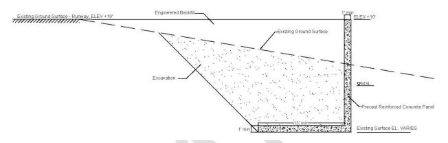
Figure 14: Alternative 5 - Precast Concrete Seawall
