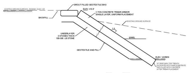
Figure 12: Alternative 2 - Tribar Revetment
