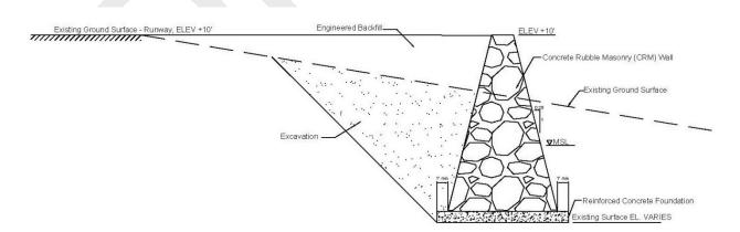
Figure 21. Alternative 3 - Preliminary CRM Wall Cross Section
