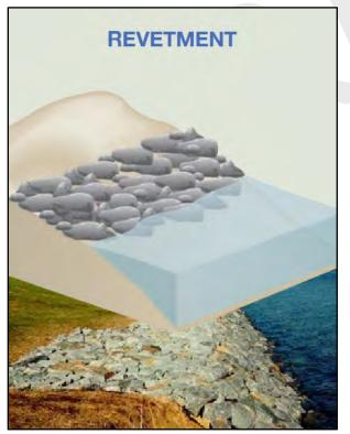
Figure 16. Revetment measure.
