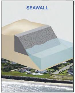
Figure 17. Seawall measure.
