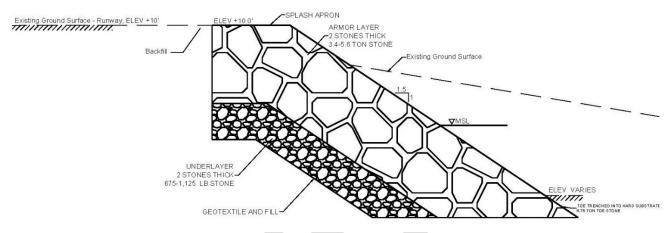
Figure 11: Alternative 1- Rock Revetment
