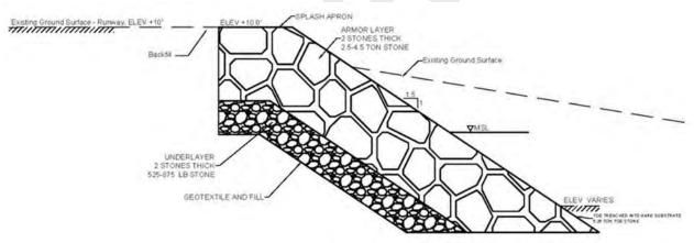
Figure 6. Preliminary Rock Revetment Detail
