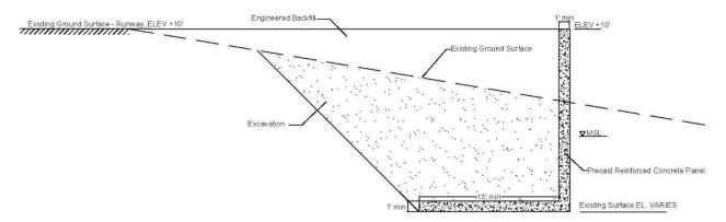
Figure 12. Preliminary Precast Concrete Seawall Detail
