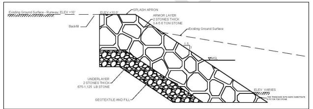
Figure 19: Alternative 1 - Preliminary Rock Revetment Cross Section
