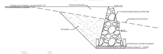
Figure 10. Preliminary CRM Seawall Cross Section Detail
