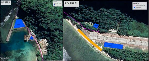
Figure 6. Staging Areas: Left: COSAs 3 and 4 in blue at Ofu Harbor. Right: COSAs 1 and 2 in blue at Ofu Airport. The tribar revetment structure is depicted in orange.
