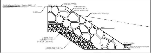
Figure 1: Alternative 1 - Rock Revetment
