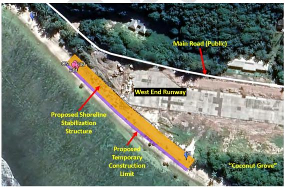
Figure 5. Project Feature Map. The orange shaded is the 0.38-acre tribar revetment (shoreline structure) to be constructed at the west end of the airport runway and the purple shaded area in
