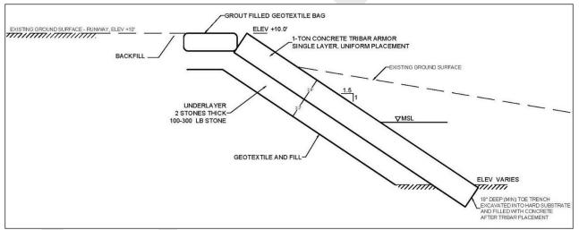
Figure 8. Preliminary Tribar Revetment Detail
